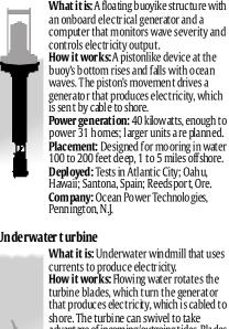
an onboard electrical generator and a computer that monitors wave severity and controls electricity output. How it works: A pistonlike device at the buoy's bottom rises and falls with ocean
